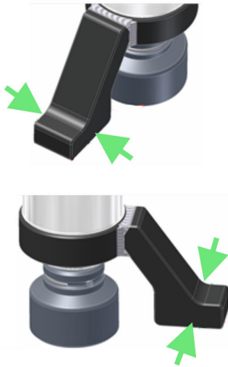
Fig. 41: Bracing the reaction arm correctly
