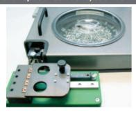
Defined pick position with integrated screw pick control option
