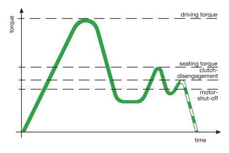
The SENSOMAT control screwdriver tightens the screw with full motor torque. Just before the base of the screw head is seated, the shut-off clutch is released and the screwdriver switches off exactly at the preset torque. The screw is completely screwed in without damaging the screw connection.
