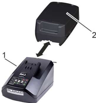
Fig. 12: Charging the battery
