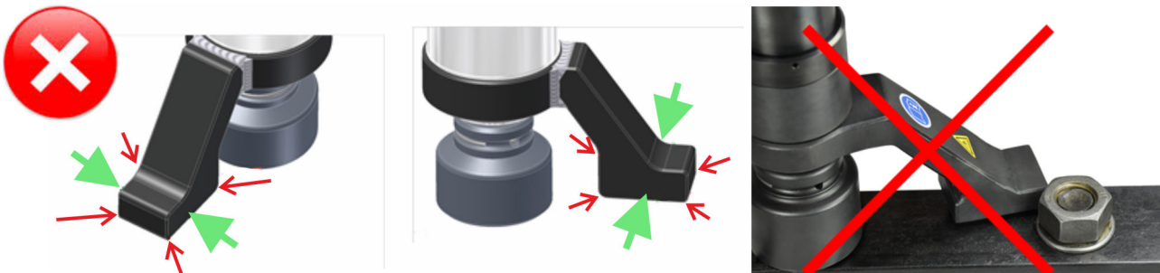
Fig. 25: Reaction arm braced incorrectly
