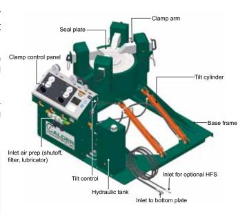
The **CALDER Recirculation Tank** offers a solution for supplying and storing fluid used for testing valves. The onboard pump supplies 3.3 gpm at 70 psi to the console. The return port on the tank allows connection to the drain line, to reclaim the fluid for the next test. The Recirculation
